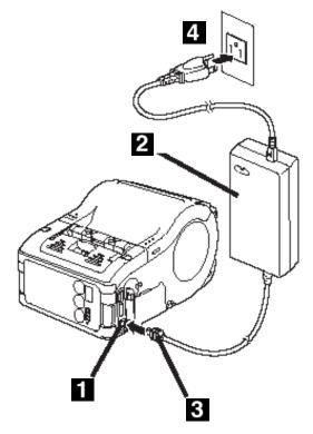
2. Connect the AC adapter to the wall outlet (4) and turn on the power.
